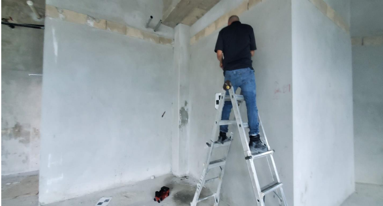
Photo 3: Performing scanning on CMU walls.
