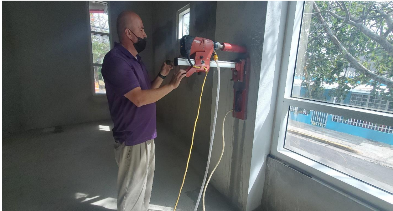
Photo 9: Core drilling to extract concrete sample for physical testing.
