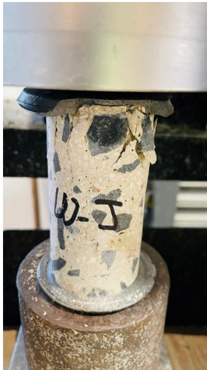
Photo 32: Core sample CO-J after testing
