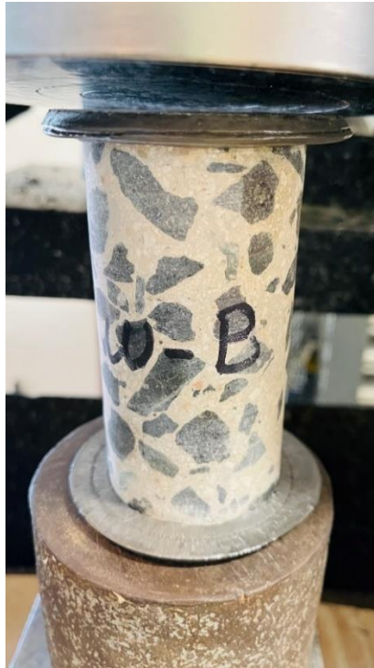
Photo 25: Core sample CO-B before testing
