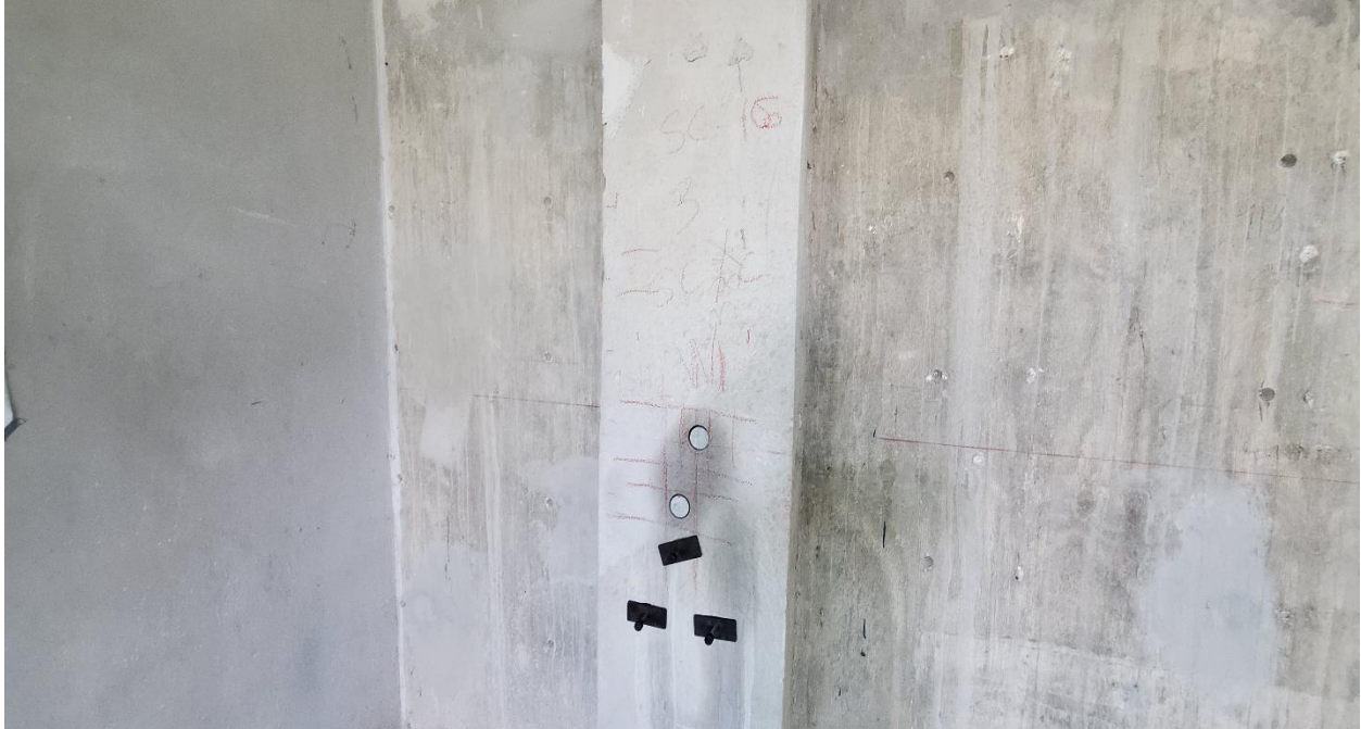
Photo 19: Windsor probes embedded into concrete columns for measuring.
