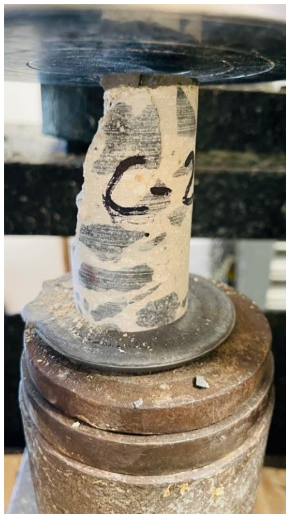
Photo 22: Core sample CO-2 after testing
