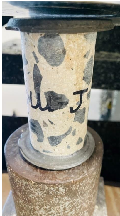
Photo 31: Core sample CO-J before testing
