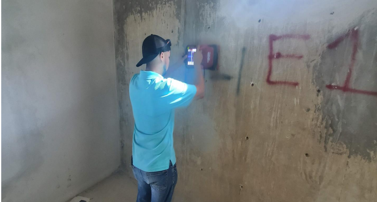
Photo 1: Performing scanning on walls before core drilling.
