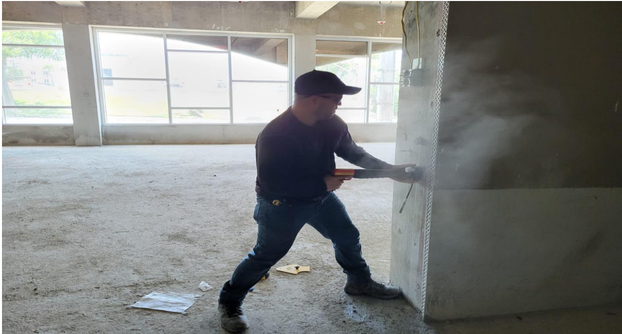
Photo 15: Performing Windsor test at columns.
