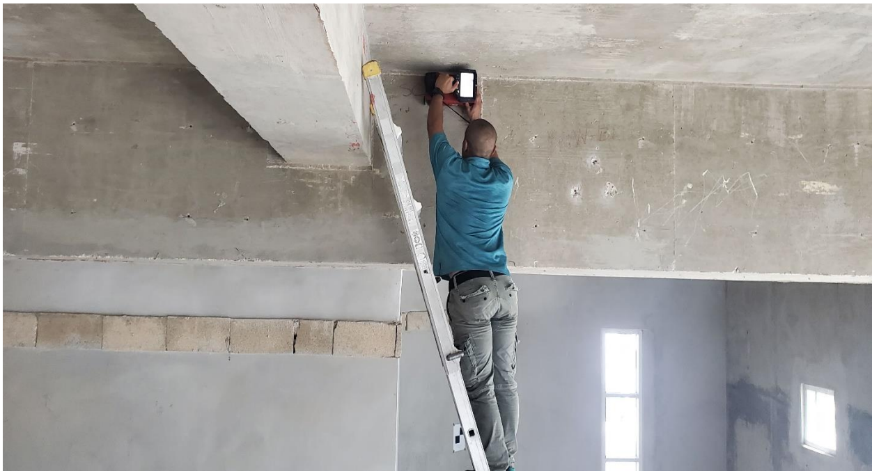
Photo 2: Performing scanning on beams before Windsor test.
