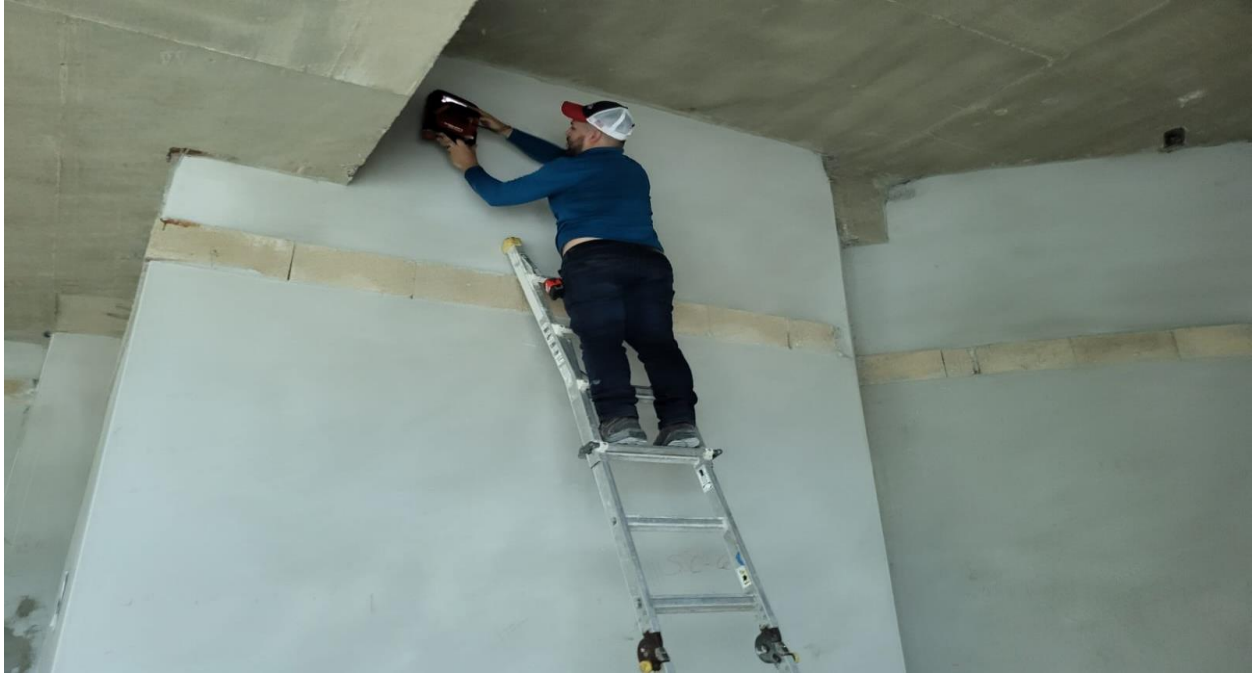
Photo 5: Performing scanning on CMU walls.
