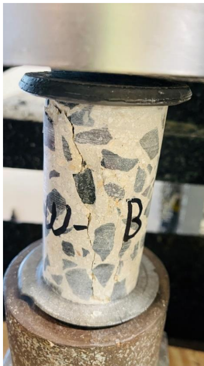
Photo 26: Core sample CO-B after testing
