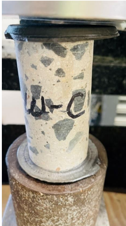
Photo 27: Core sample CO-C before testing
