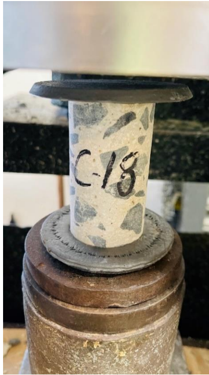
Photo 23: Core sample CO-18 before testing
