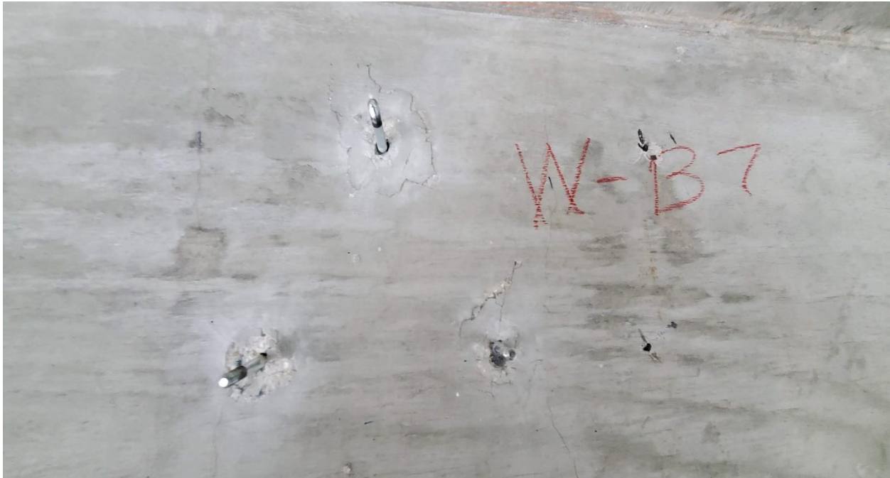
Photo 17: Windsor probes embedded into concrete beams for measuring.
