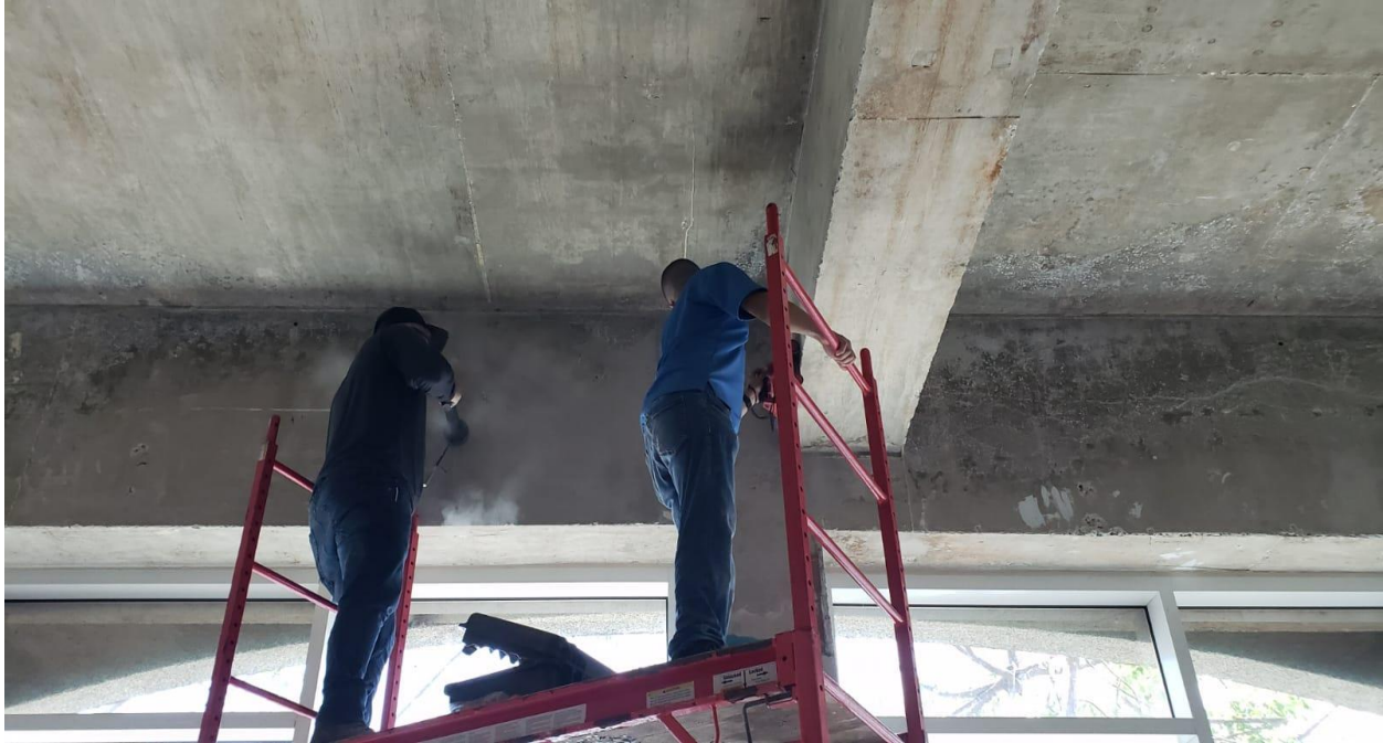
Photo 7: Scanning beams to determine the reinforcement.
